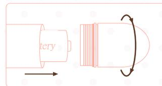
Remove the end cap by turning it anticlockwise. (The Golden Bar will be turned on for a moment during the process). Withdraw the battery from the tube.
